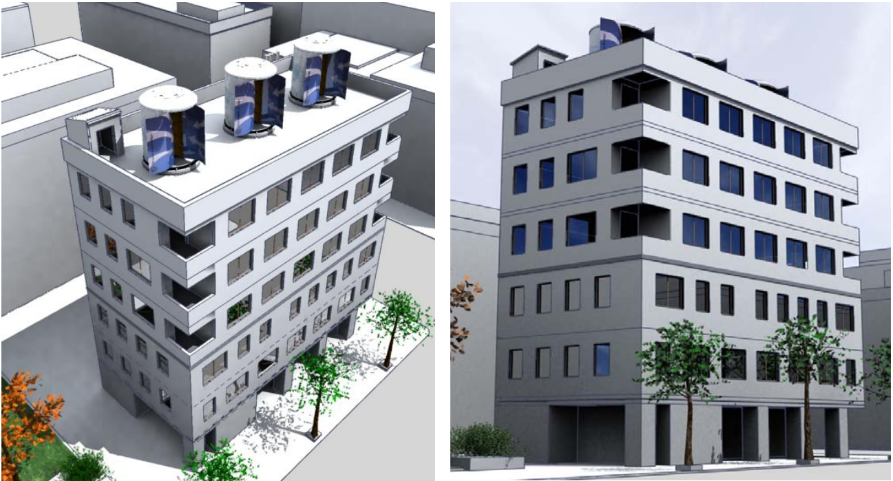
Figure 20: Apartment building with an installation of three Hammurabi 5kW
