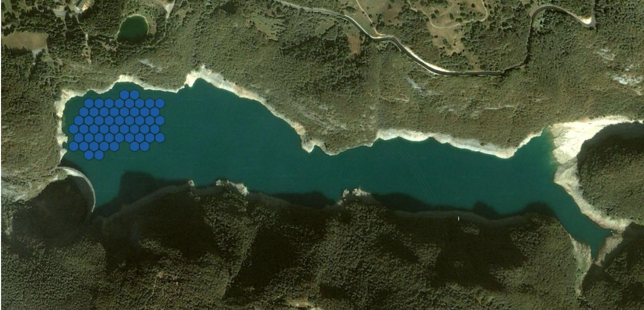
Figure 7 Speccheri basin: scheme of a 3 MWp FTCC plant.
